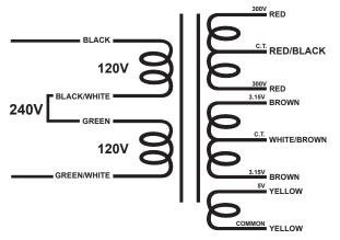
120 Volt Primary: Connect the two primary windings in parallel.
