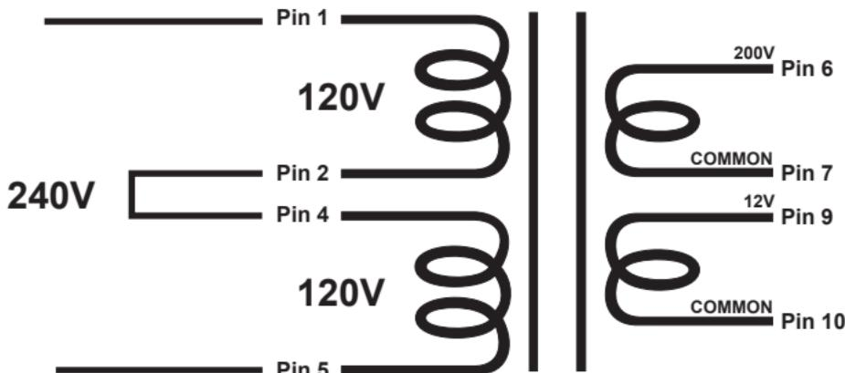
**120 Volt Primary:** Connect the two primary windings in parallel.
