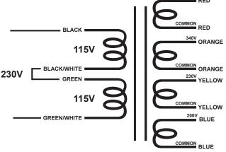
**115 Volt Primary:** Connect the two primary windings in parallel.
