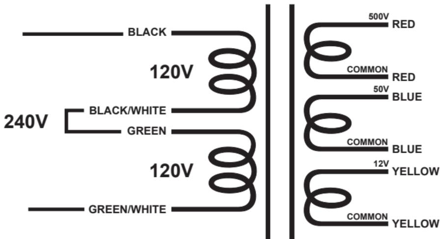
**120 Volt Primary:** Connect the two primary windings in parallel.
